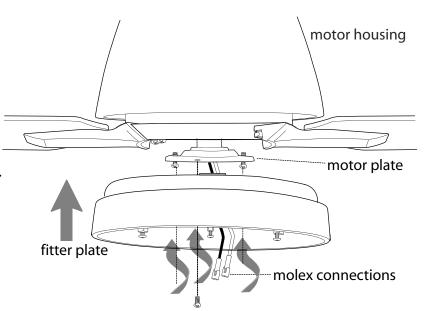
Remove 1 screw from post located on underside of fitter plate and partially loosen the other screws in the other two posts.
