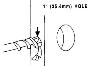
Drill 1" (25.4mm) hole in center of door edge for latch.
