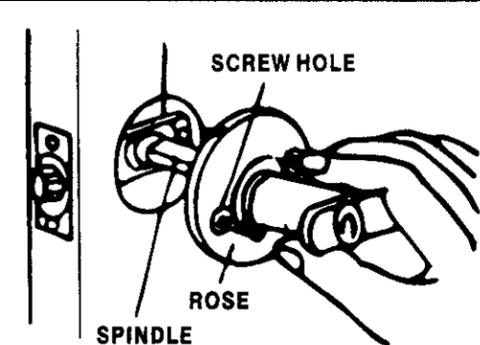
Install interior lever and rose by placing spindle through rose hole and aligning screw holes with stems. Push flush against door. Insert screws and tighten until lockset is firm.
