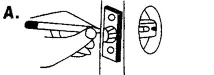
Insert latch in hole, keeping it parallel to face of door. Mark outline and remove latch
