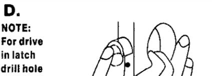
**NOTE:** For drive in latch drill hole 1" (25.4mm) and press latch until it is flush with door edge
