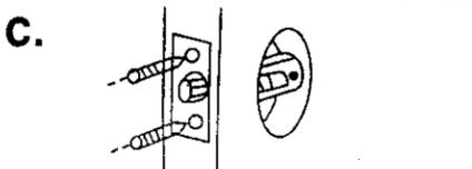
Insert latch and tighten screws.
