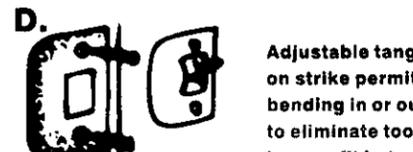
Adjustable tang on strike permits bending in or out to eliminate too loose a fit between door and door stop. Install strike and tighten screws
