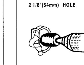
Drill 2 1/8" (54mm) hole through door face as marked for lockset. It is recommended that holes be drilled from both sides to prevent splitting.
