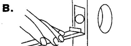
Chisel 1/8" (3mm) deep or until latch face is flush with door edge.
