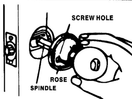
Install interior knob and rose by placing spindle through rose hole and aligning screw holes with stems. Push flush against door. Insert screws and tighten until lockset is firm
