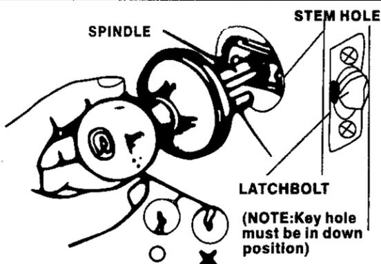
Insert knob of lever with spindle into latch, making certain that stems are positioned correctly through stem holes. Press flush against door
