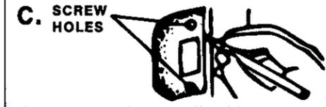
Match screw holes on strike with center line on jamb. Outline outside edge of strike. Chisel 1/16" (1.6mm) deep for strike.
