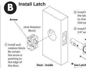
② Install latch and rotate the latch tongue \*\* to change handing. (See page 1 for handing)
