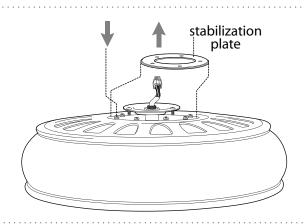
**Tip**: To prepare for threading electrical wires through downrod, apply a small piece of electrical tape to the ends of the electrical wires--this will keep the wires together when threading them through the downrod.
