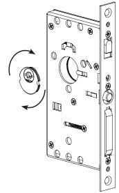
Note: Notches on cylinder must be parallel with the horizontal plane when fully screwed into lock body.
