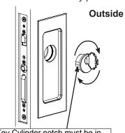
Key Cylinder notch must be in the horizontal position when fully screwed in lock body.
