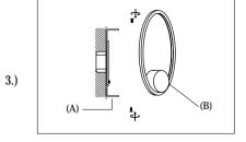
Step 3:Install Body (B) to Canopy (A) and tighten screws on the sides of the canopy to secure.
