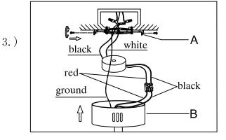
Step.3: Wire low voltage red/black wires to the terminal block, and wire high voltage black/white wire to the outlet box. Install the canopy (B) to the mounting bracket (A) using screws provided.
