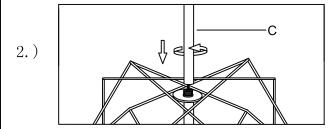
Step.2: Run wire through stem (C) lengths and combine stem lengths to meet desired mounting height. Attach the stem (C) to the body of the fixture.
