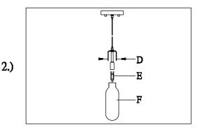
Step.2. Insert the G9 bulb(E) into socket
