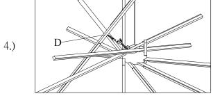
Step.4: Using the quick connect plug, wire the LED arm (D) to the fixture body. Secure to the body of the fixture using screws provided.
