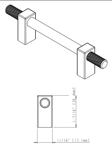
ACCESSORY: SCREW:8-32XI" 2PCS BREAK AWAY SCREW:8-32x45 2PCS ALL SCREW MATERIAL: STEEL-SAE1006
