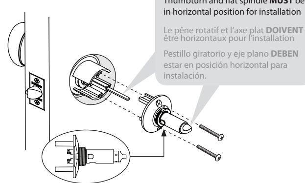
Thumbnut and flat spindle **MUST** be in horizontal position for installation
