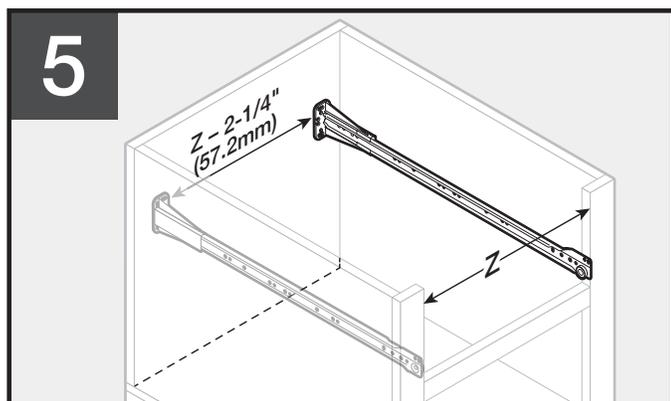
**5** Repeat Steps 3-4 for remaining cabinet member. Measure cabinet opening; subtract 2-1/4" (57 mm) for distance between rear sockets.
