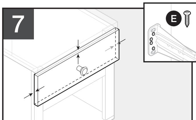
**7** Check alignment of drawer relative to the cabinet. Remove drawer and adjust sockets (F & G) if necessary. Once final placement is achieved, secure sockets with remaining screws (E).
