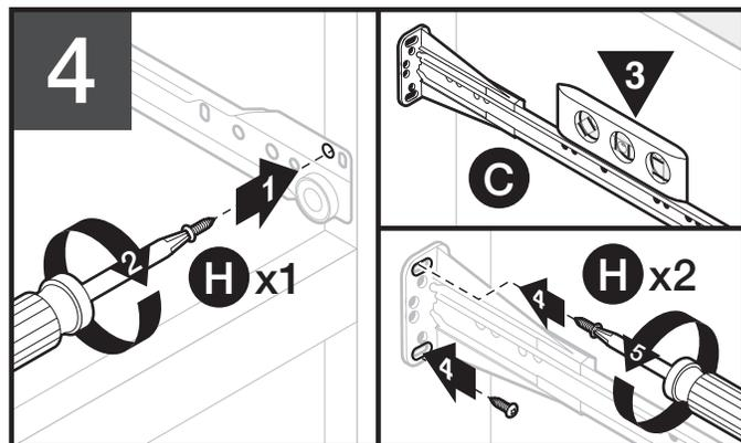
**4** Secure front of cabinet member with a screw (H). Make sure cabinet member (C) is level; secure right socket (G) with screws (H).
