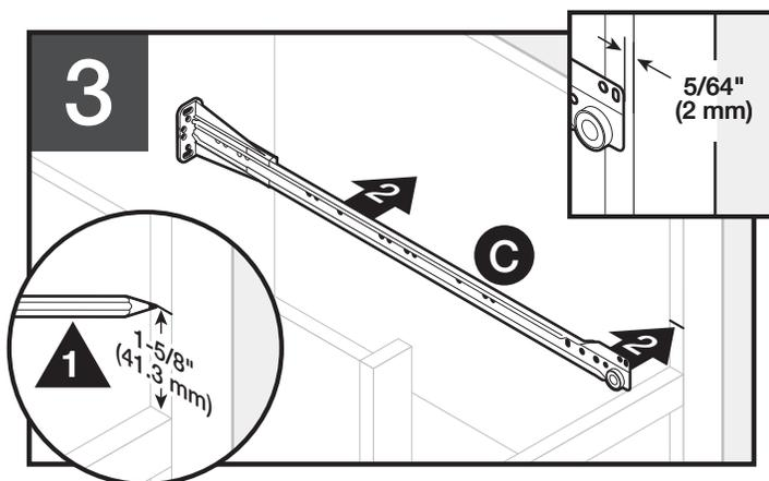
**3** Mark 1-5/8" (41 mm). Align top of cabinet member (C) with mark, 5/64" (2 mm) from front of cabinet.
