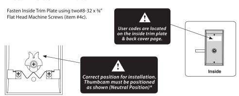
\*Neutral position is required for installation and removal of the Inside Trim Plate Assembly.
