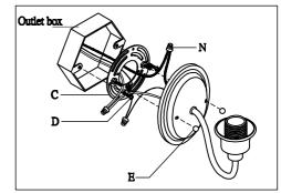
Step 1. Remove mounting bracket (C) from fixture and install to electrical box. Then wire fixture to wires in outlet box. Copper wire is for Ground.
