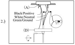
Step2: Adjust wire length to desired mounting height, and tighten strain relief screws to secure. Wire fixture to wires in outlet box. Green wire is for Ground.
