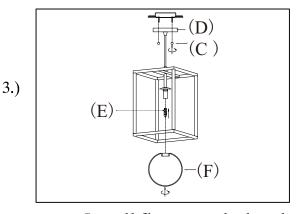
Step3: Install fixture to the bracket using ball nuts on the canopy. Install bulb provided into socket and thread the glass onto socket.
