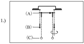
Step1:Remove mounting bracket from fixture and install to electrical box.
