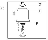
Step.3: Place glass over socket and secure using threaded socket cover (F). Use Max 60W bulbs.
