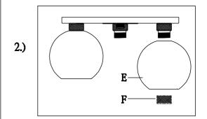
Step2: Attached the Glass(E) to the socket, then secured by socket ring(F)
