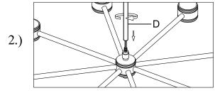
Step 2: Run wire through stem (D) lengths and combine stem lengths to meet desired mounting height.
