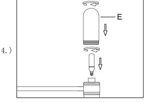
Step.4: Install 40 Watt candelabra base bulb. Then, Thread glass (E) into fixture.
