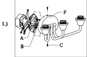
Step.1: Remove mounting bracket (A) from fixture and install to electrical box.
