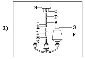
Step .2: Attached the glass(F) on the socket, then secure by socket ring(G).
