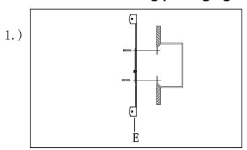
Step. 1: Install mounting bracket (E) to outlet box.
