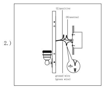
Step. 2: Wire fixture to wires in outlet box. Copper/green wire is for Ground.
