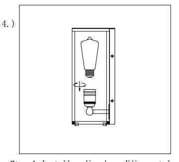
Step. 4: Install medium base Edison-style bulb (not included) into socket.
