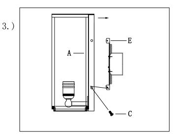
Step. 3: Run a bead of silicone sealant along the edge of the backplate to prevent water intrusion. Leave a gap at the bottom to allow moisture to escape. Attach the fixture to the mounting bracket(E) using screws(C) provided.
