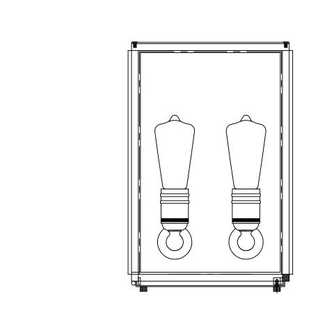
CAUTION: To prevent water intrusion, caulk around back-plate where fixture meets the wall using outdoor silicone sealant. Leave a small gap at the bottom to allow moisture to exit.
