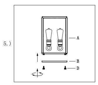
Step. 5: Attach bottom cover(B) to the body(A) and tighten screws(D) on the bottom of the fixture to secure.
