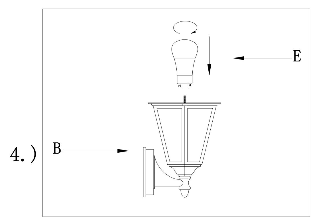
Step.4: Install GU24 LED bulb(E)
