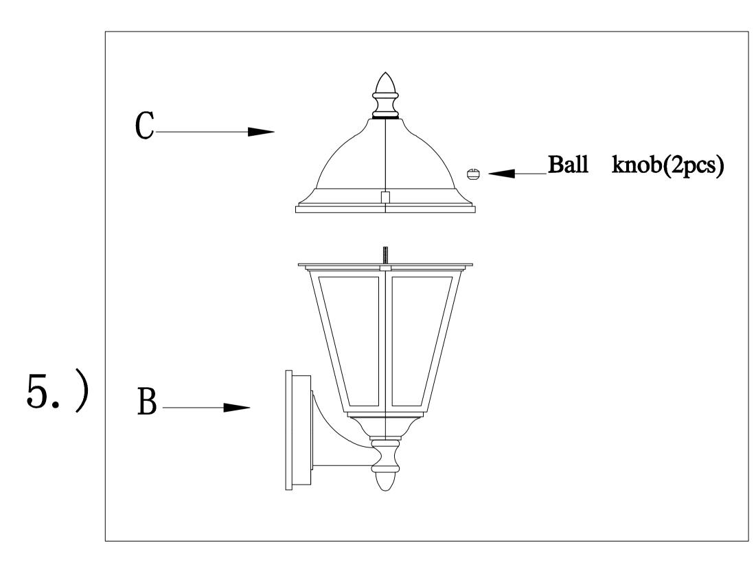
Step.5: Lnstall cover(C) to fixture, using ball knobs.
