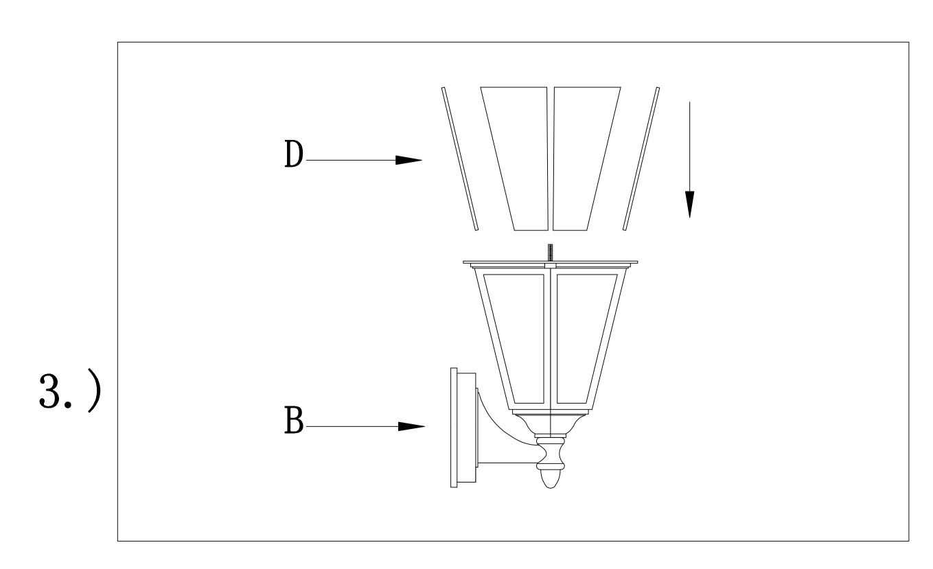
Step.3: Install the sheet glass(D) into the fixture(B)
