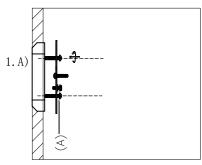
Step.1 Remove mounting bracket from fixture and install to electrical box.
