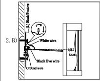
Step.2 Wire fixture to wires in outlet box.
