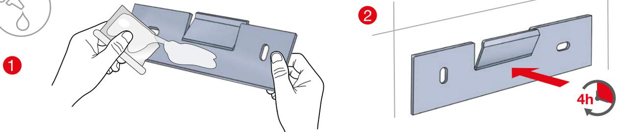
**!** EN We recommend i.Composite GlueMix. Carefully clean the surface to be glued. It is important to follow the glue manufacturer's instructions. See also attached mounting instructions. Not recommended for mounting on any wallpaper. Glue to be bought separately.
