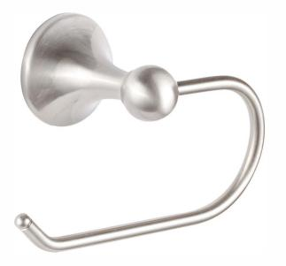
Post materials: zinc Towel bar tube material: brass 3" extension from wall 2 1/8" base Concealed screw mounting with straight standard head fixing screw Plated steel mounting brackets with two screws each
