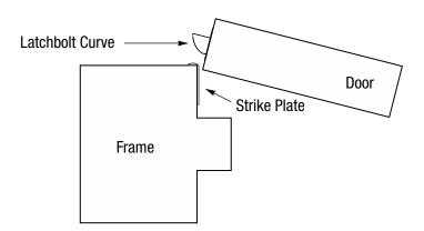
Curve of latchbolt must contact strike plate first.
